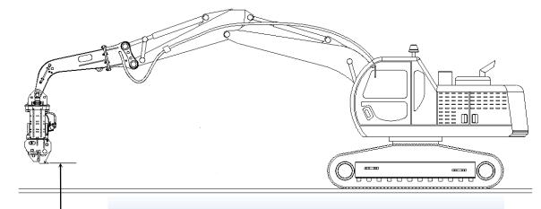
Extension boom with **JOINT**, W250 can be used up to **8M** of increased driving height
